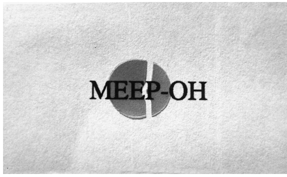
Figure 3 Photograph of a disc of a hybrid with a MEEP-OH:SiO 2 = 0.8 and a thickness of 120 μm.
